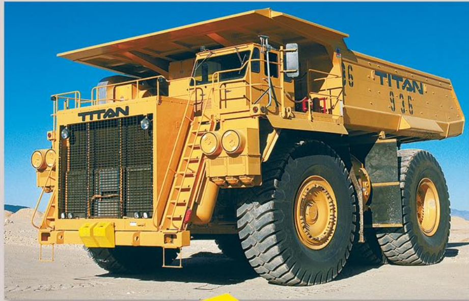
Marathon Le Tourneau Titan 2000 Series Haul Truck With Model 1900 Mounting Bracket And Two Model 1812 Checkers Roadblock Wheel Chocks Mounted On Front Bumper.
